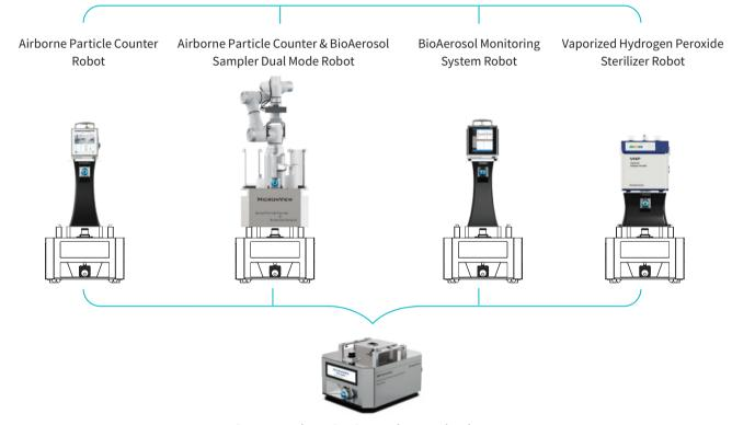
**Environmental Monitoring and Control Robot Base**
